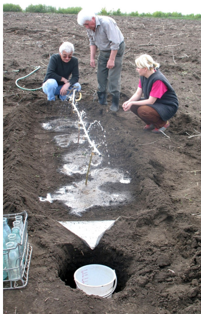
Fig. 1. Determining the volume and turbidity leaks under the influence of artificial rain of certain intensity
